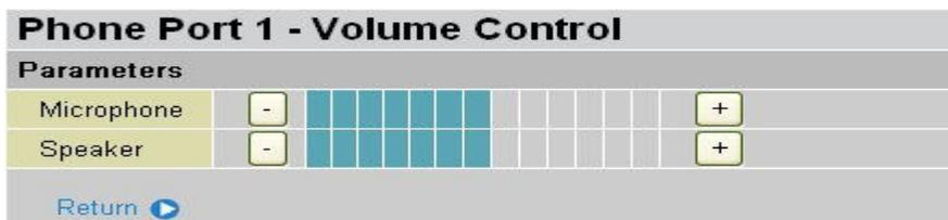
Volume control helps you to adjust the sound level of the telephone to the best comfortable listening level. Echo problems can be caused by having the levels set too high.
