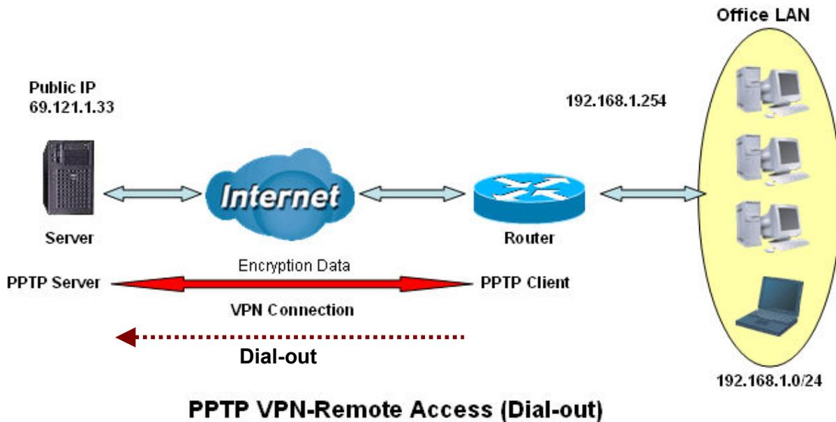
**Example: Configuring a Remote Access PPTP VPN Dial-out Connection (ctd)****Configuring the PPTP VPN in the Office**
