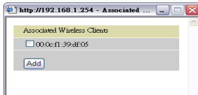
Associate Wireless Client displays a list of individual wireless device MAC Address that are currently connected to the router. Select the required device to be blocked or allowed by checking the box next to the MAC Address. Then click **Add** to insert to the Wireless Client (MAC Address) Filter table. The maximum number of Wireless clients filter entries is 16.
