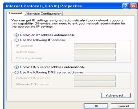
Figure 3.4: IP Address & DNS Configuration
